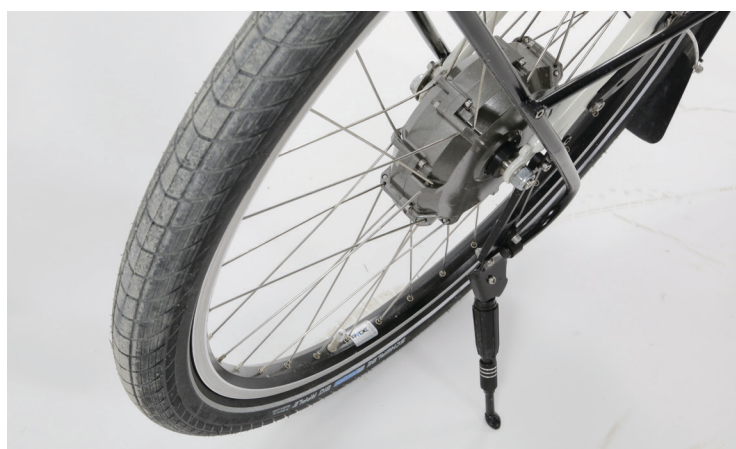
LEFT The front wheel motor has a housing from Chinese manufacturer Crystalite, but according to Utopia the internals, windings and electronics are all made in the Netherlands.
